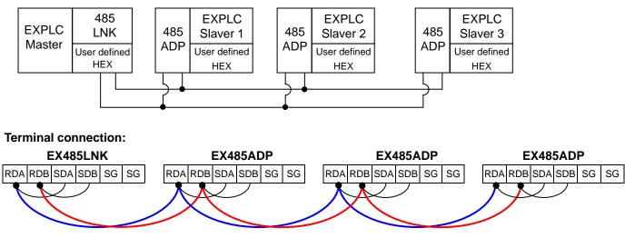
♦ At this mode, please set communication format to without STX, ETX1 and ETX2, 8 bits Even Parity, Stop bit 1. Transmission speed and communication format of master and slave have to be the same. Transmission format is defined by user.
