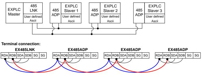
♦ At this mode, please set communication format to with STX, ETX1 and ETX2, 7 bits Even Parity, Stop bit 1. Transmission speed and communication format of master and slave have to be the same. Transmission format is defined by user.
