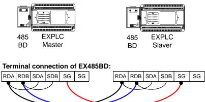
**Note:** The version of two PLCs (Master and Slaver) must be the same, i.e., the contents of D8001 of two PLCs are the same.
